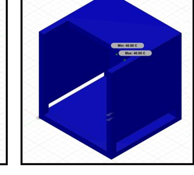
EPA filters were selected for their high efficiency in removing particles as small as 0.3 microns, while activated carbon filters were chosen for their ability to adsorb volatile organic compounds (VOCs) and other harmful gasses. As cool air enters through the bottom, it passes through the filters, removing pollutants before circulating up and out through the top of the incubator.
