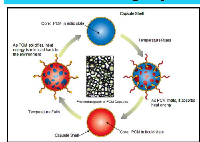
Phase change materials are substances that absorb and release large amounts of energy when they transition between different physical states, like solid and liquid, at a nearly constant temperature, making them useful for thermal energy storage and management.
