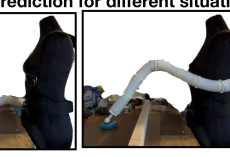
Touching Object, "Touch" Speech Command. This movement goes around the right of the body. Object avoidance, No speech Command. Goes around the left side of the body for curl
