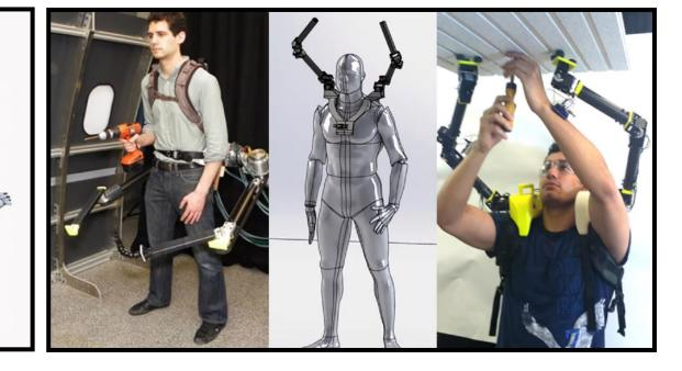
Rather than replacing existing limbs like exoskeletons and traditional prosthetics, SRLs are additional limbs attached to the user's upper body, designed to enhance functionality rather than restore lost movement. SRLs function independently, allowing users to perform tasks they could not achieve with their natural limbs alone.
