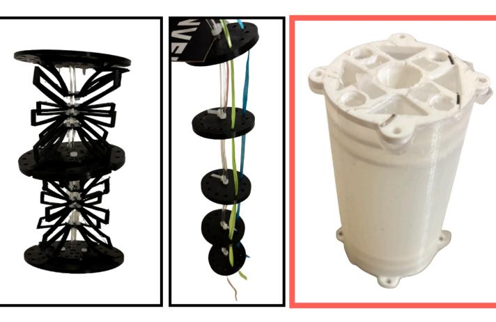
Prototype 1: Continuum arm modeling a human spine, using rigid vertebrae and air tubing.
