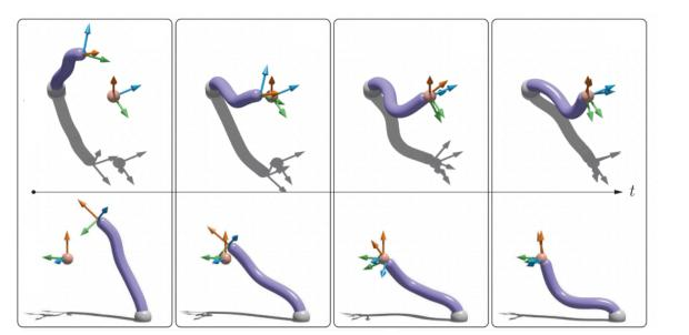
Path progression to a randomized point The 3-segmented continuum arm makes its progression toward the point and its subsequent reorientation. Fixed to a predetermined origin.
